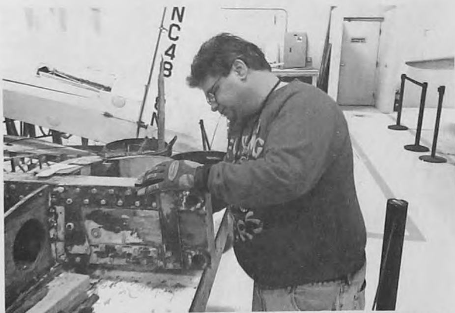
Chris Curran of Allen Park scrapes paint metal parts on the wing where it attaches to the fuselage.
